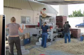
REACCH graduate students processing biomass samples using a Vogel stationary thresher.
