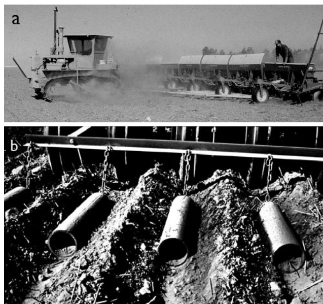
Fig. 16. (a) Development of the deep-furrow split-packer John Deere HZ drill in the mid-1960s was a major advancement for winter wheat–summer fallow farming because seed could be placed up to 18 cm below the surface into moist soil. This allowed farmers to establish wheat early (late August to early September) for optimum grain yield potential. (b) Deep furrows spaced 41 cm apart help minimize the soil cover over the seed, but winter wheat seedlings still have to elongate through 10 to 15 cm of soil to reach the surface. The drags behind the drill are sometimes used to help stabilize the furrow and reduce the thickness of soil covering the seed. Photos by W.F. Schillinger.
