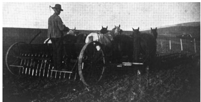
Fig. 9. An early model hoe grain drill with rows spaced 20 cm apart. Seed was dropped through rotating flutes in the seed box down tubes behind the openers to the soil surface. Chains were attached behind each tube to lightly cover the seed with soil. Photo from Brumfield (1968).
