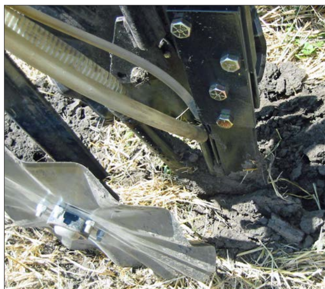
Figure 5. Fertilizer application components (hoses) mounted on a tillage shank.
