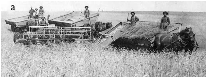
Fig. 5. (a) Cutting and loading wheat in the field with a header into a header wagon for transport to a threshing site. The header is equipped with a reel that lays the wheat stalks across a reciprocating sickle bar for cutting standing grain and onto a canvas platform for elevating into the wagon. It is ground driven, cuts a swath 3.5 to 6 m wide, and is pushed from the rear by six horses. Photo courtesy Terry Olson family, Ritzville, WA. (b) Stationary threshing. The wheat spikes and straw on the header wagon lay on a rope netting that holds the load together as it is lifted off by the derrick with a rope and pulley and dropped beside the thresher. From there it is hand pitched into the thresher that separates the grain from straw with grain fed into sacks and the straw blown into a pile. The thresher is belt powered by a steam engine that burns wheat straw. This mode of harvesting required up to 30 men to operate and was common during the last decades of the 1800s and was replaced by the combine in the early 1900s. Photo from Northwest Museum of Arts and Culture, Spokane, WA, L83-113.48.
