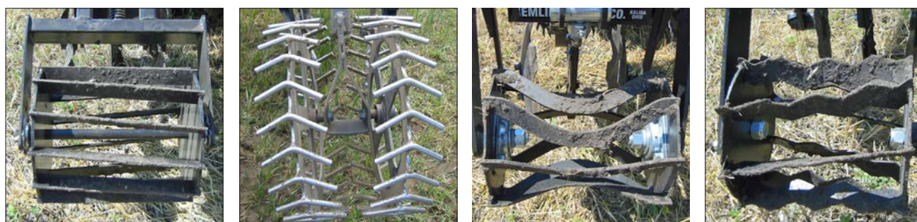
Figure 6. Soil conditioners used on strip-till implements are available in many shapes and sizes for the wide variety of soil types and desired conditions.
