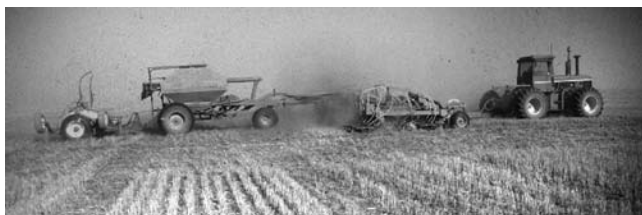
Fig. 18. A modern Flexi-coil no-till drill delivers seed and fertilizer in one pass through the field. This 11 m wide drill has an attached tank cart that carries seed in one section and granular starter fertilizer in the other section. Aqua \text{NH}_3\text{-N} , carried in the 3800-L tank at the end, is pumped forward and delivered slightly to the side and below the seed. Photo by W.F. Schillinger.
