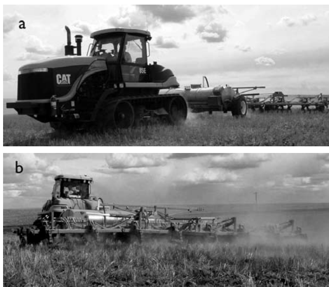
Fig. 19. (a) A modern 375-horsepower Caterpillar 85E crawler tractor pulls a 3800-L tank filled with aqua \text{NH}_3\text{-N} , and a Haybuster undercutter during primary spring tillage plus N fertilizer injection near Lind, WA. The 11 m wide implement is operated at 10 \text{ km h}^{-1} and covers about 75 \text{ ha d}^{-1} . The tank needs to be refilled with aqua \text{NH}_3\text{-N} every hour. (b) The wide, narrow pitch, and overlapping V-blades on the undercutter implement slice below the surface with little soil lifting or disturbance of surface residue, but completely sever soil capillary continuity to halt upward movement of liquid water to maintain seed-zone moisture in summer fallow. Note the standing stubble that is much more effective than flattened stubble for wind erosion control. This represents the best technology currently available for profitable and environmentally sound winter wheat–summer fallow farming in the low-precipitation zone of the Pacific Northwest. Photos by W.F. Schillinger.
