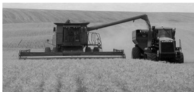
Fig. 20. A new John Deere 9760 level-land combine with 10-m header unloads wheat on the go near Ritzville, WA, in July 2006. The grain yield of soft white winter wheat in this field averaged 3220 \text{ kg ha}^{-1} . The combine operated at a speed of 8 \text{ km h}^{-1} and harvested 6.7 \text{ ha h}^{-1} . Farm machinery costs have skyrocketed in recent decades. This combine was rented from an equipment dealer for \$150 \text{ separator h}^{-1} . The price of a new machine is \$250,000 . Photo by Derek Schafer.
