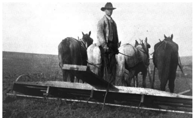
Fig. 8. A stationary (i.e., nonrotating) rodweeder that had two rods spaced 1 m apart. By walking forward on the plank, the driver tilted the front rod down underneath the soil as seen here. When the front rod became plugged with weeds or residue, the driver stepped to the end of the plank to bury the second rod and raise and clear the first rod. The driver needed to tilt the rodweeder back and forth several hundred times during the day. Plugging during rodweeding was eliminated with the introduction of the rotating rodweeder in 1907 (see Fig. 10). Photo from Brumfield (1968).
