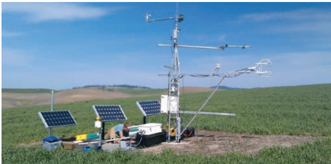
Eddy covariance tower to continuously measure the exchange of \text{CO}_2 over a wheat field.
