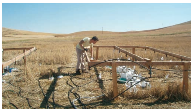
Automated static chambers monitor subsequent greenhouse gas emissions on micro-plots. Photo by Dave Huggins.
