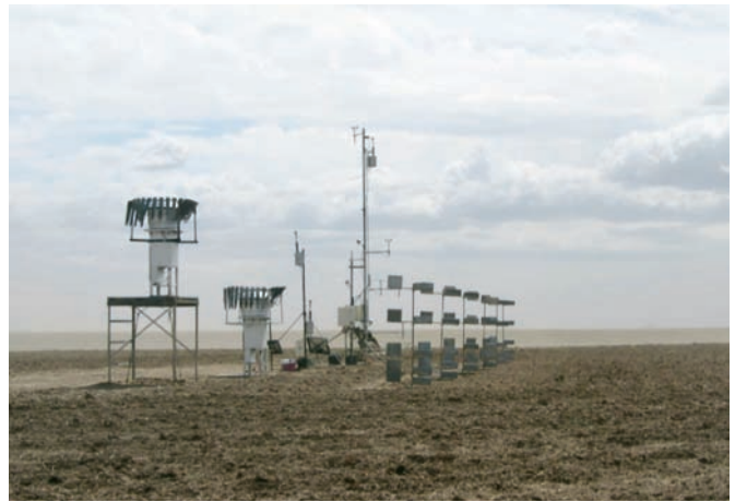
Nitrogen loss from agricultural fields during high wind events was assessed using a series of profile samplers that trapped windblown dust; the profile samplers are located to the right of center in the photo.
