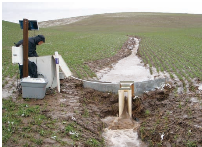
Carbon export through surface runoff was monitored using parshall flumes and event-based water sampling. The image above was taken at the conventional tillage site.
